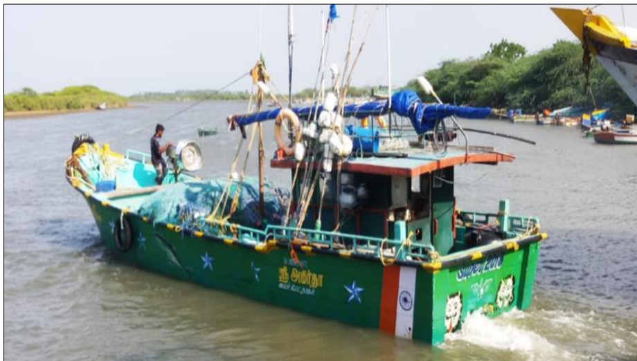
Bottom Trawler converted into Tuna Long Liner
